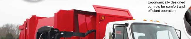
A 35" straight vertical lift before the cart tips allows for easy collection off of retaining walls and snow banks.
