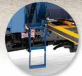
Folding ladder allows for convenient hopper access.
