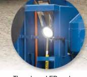
Three large LED work lights provide ample illumination.
